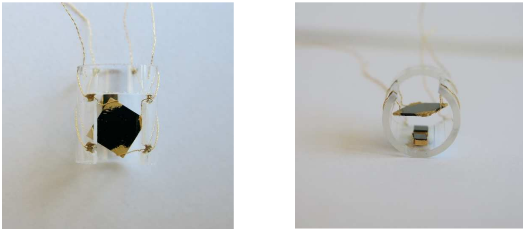
Fig. 3.1: Sample in van-der-Pauw geometry mounted inside a quartz-glass holder (left: top view, right: side view).
