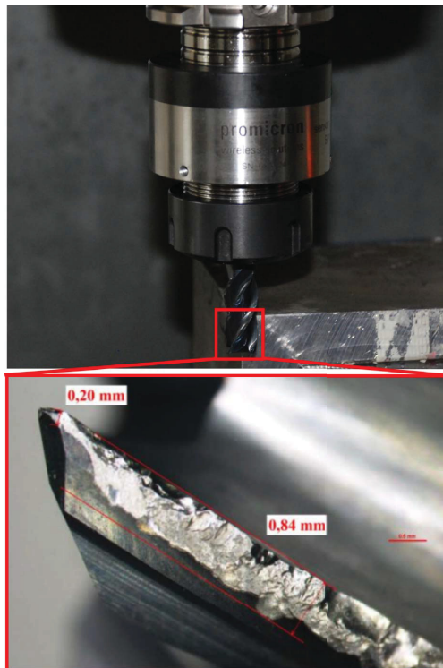
Fig. 1: The instrumented chuck is equipped with four strain gauges, enabling the measurement of: bending moments M_x and M_y in orthogonal direction; the torque T and the holding force F_a . In addition, there is a temperature sensor. The chuck is also equipped with a wireless data connection to enable a remote real-time observation of the measured values. The magnification shows the damage of one cutting edge at the end of the life time experiment.
