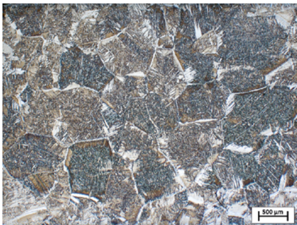
Fig. 2: 3% \text{HNO}_3 etchant revealing the PAGs after solution annealing of a quenched 0.17% plain carbon structural steel.
