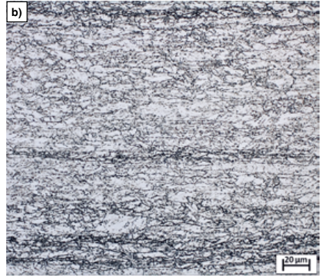
Figs. 4a to c: a) TM-UHSS 1 etched with modified etchant using sodium dodecyl sulfate as wetting agent, composition according to Tab. 2, b) TM-UHSS 1 with refined microstructure, the etchant even reveals grain sizes < 1 \mu\text{m} c) TM-UHSS 2 etched with picric acid and wetting agent, dispensed with HCl.
