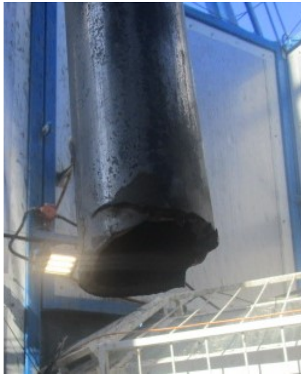
Figure 12: The photo of broken drill pipe (NWDP 88,9 x 9,35 G-105)
