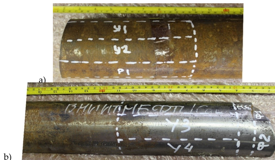
Figure 23: Sample marking for endurance limit test. a) Fragment #1, b) fragment #2
