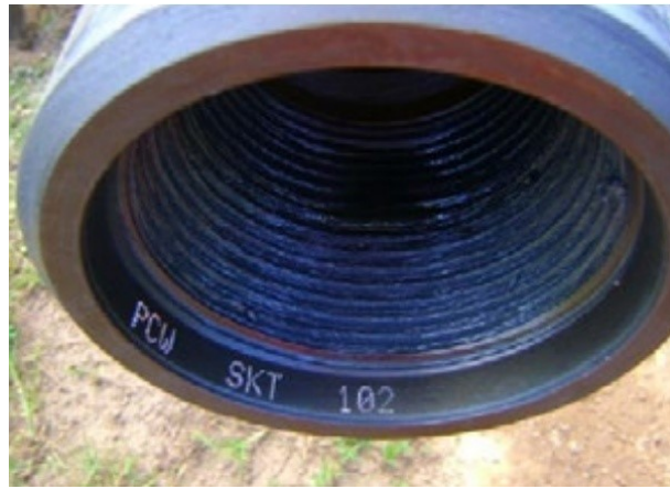
Figure 38: Marking space for drill pipe tool joint
