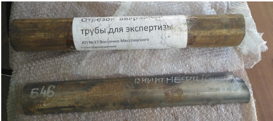
Figure 18: Two pieces of broken pipe delivered for the expertise
