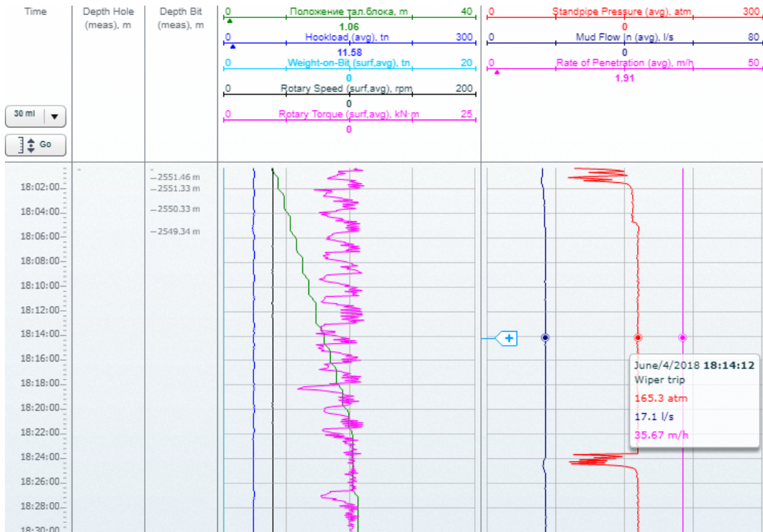
Figure 25: Mudlogging data screenshot. Wiper trip operation from 18:00 to 19:30 (04.06.18)
