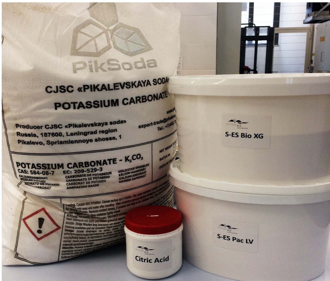
Figure 45: Ingredients for the water-based K_2CO_3 drilling mud
