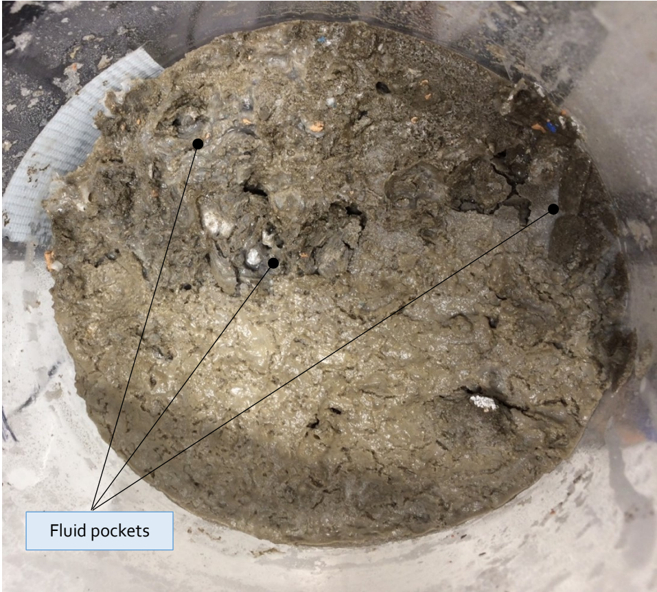
Figure 57: Mud pocket contaminated kick-off plug (top view)
