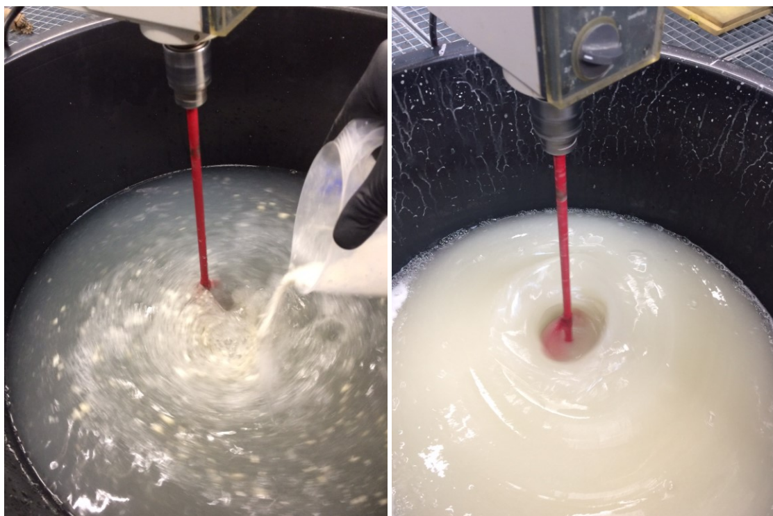
Figure 46: Preparation of the drilling mud
