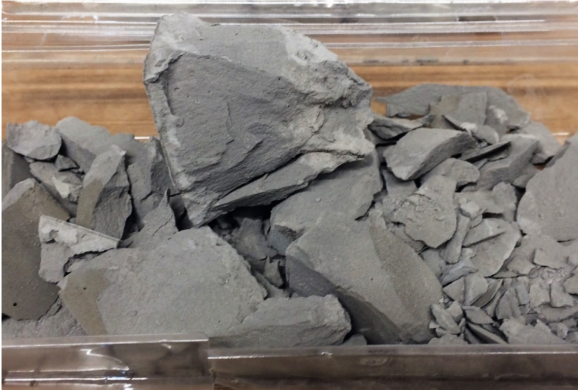
Figure 80: Neat Class G sample after testing procedure
