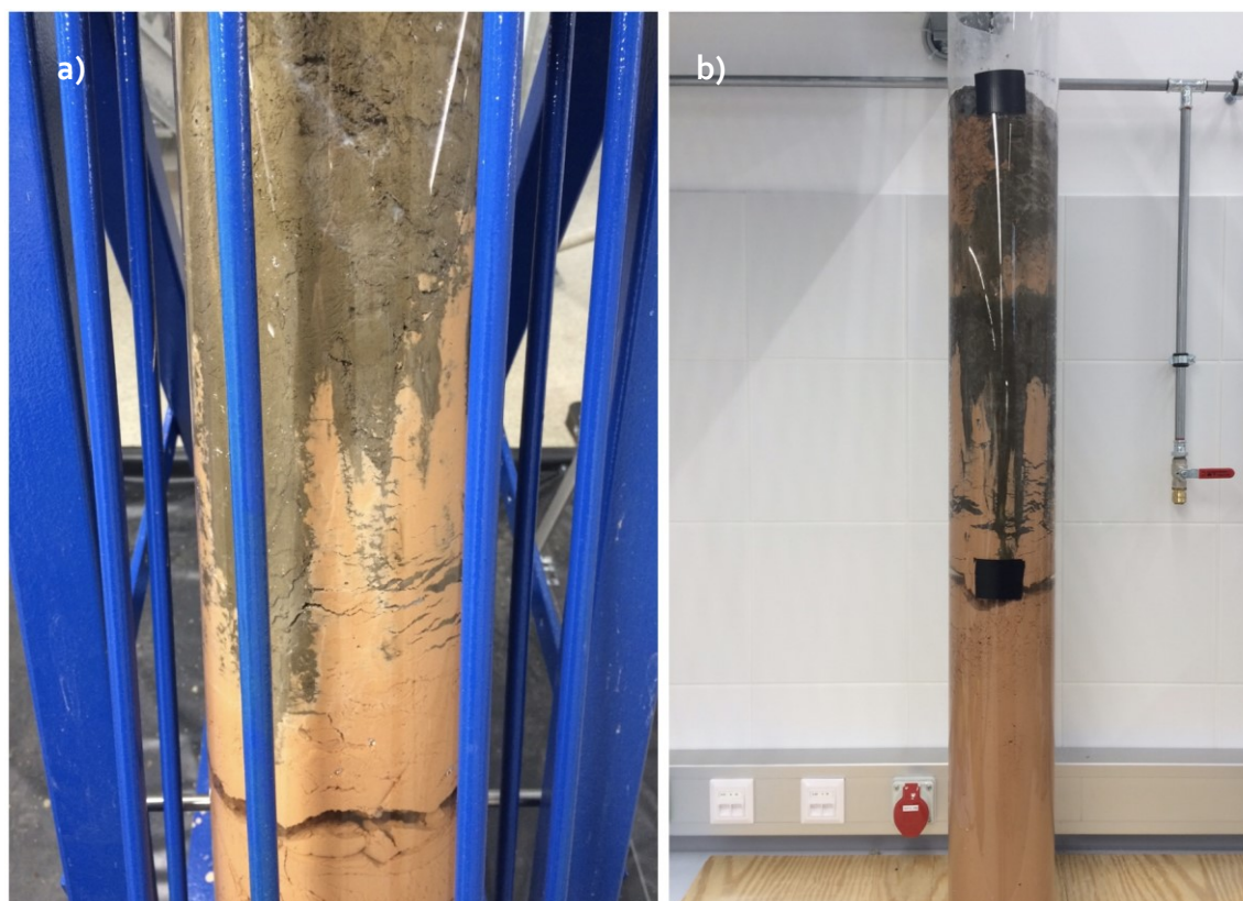
Figure 56: Kick-off plug partly falling through the plug base
