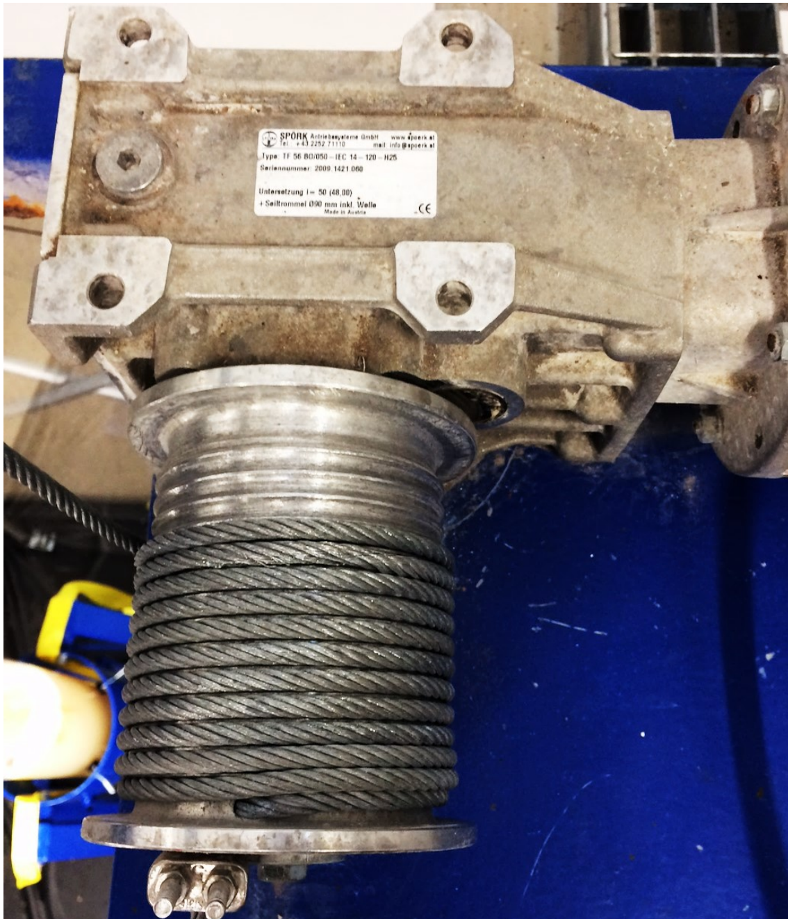
Figure 39: Lebus groove system of the drawworks drum
