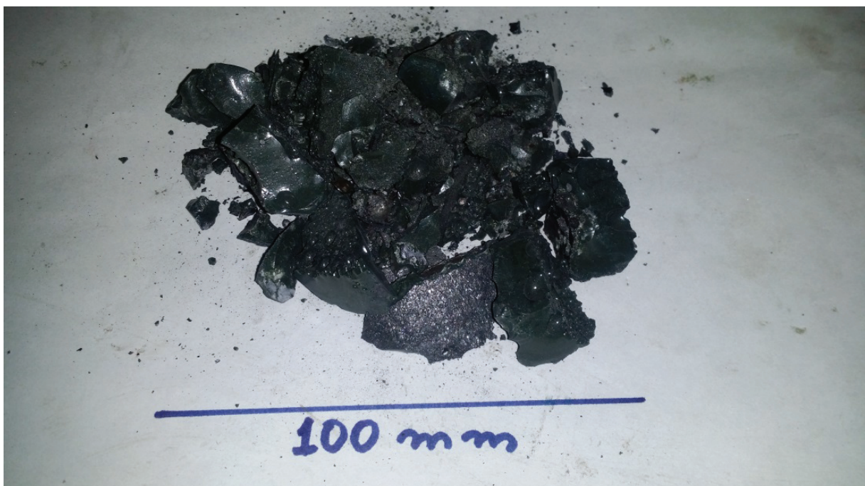
Figure 7-9: Melted non-metallic Content of Recuperated Scrap
