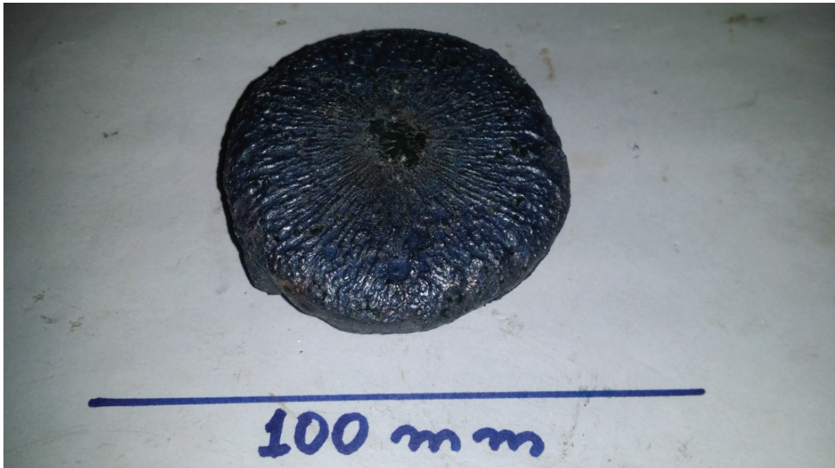
Figure 7-8: Melted Metallic Content of Recuperated Scrap
