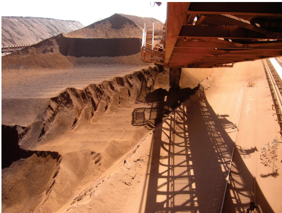
Figure 2.8: Trench cutting operation (courtesy of Sandvik)
