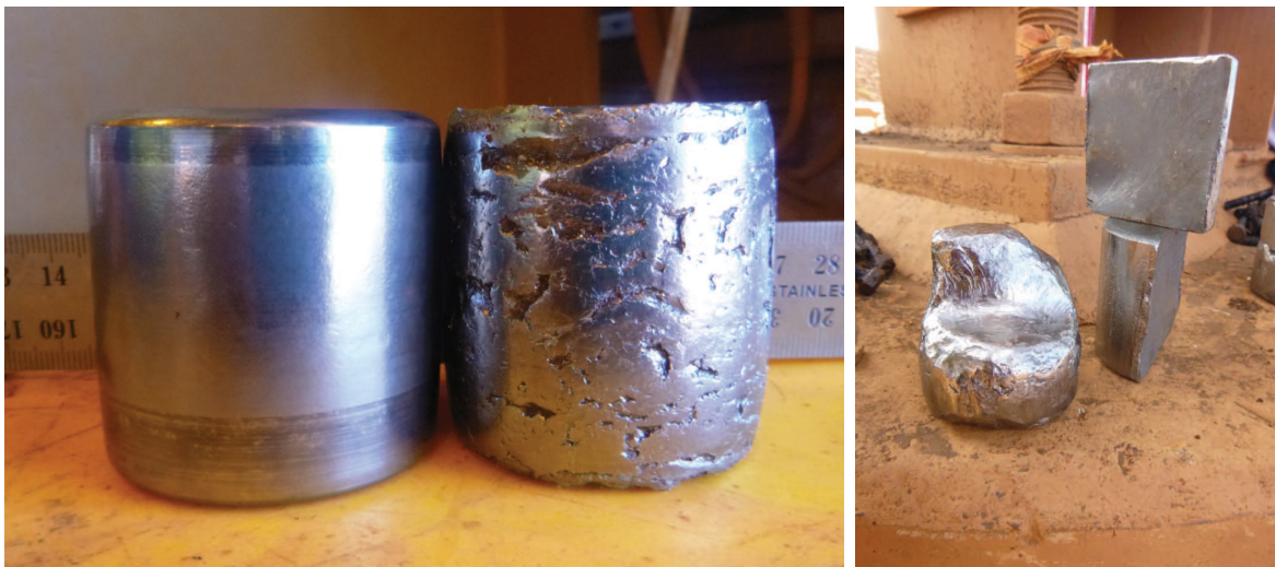
(a) Roller elements of the same slew bearing - Left element with slight wear, right element with excessive damage (b) Broken roller elements
