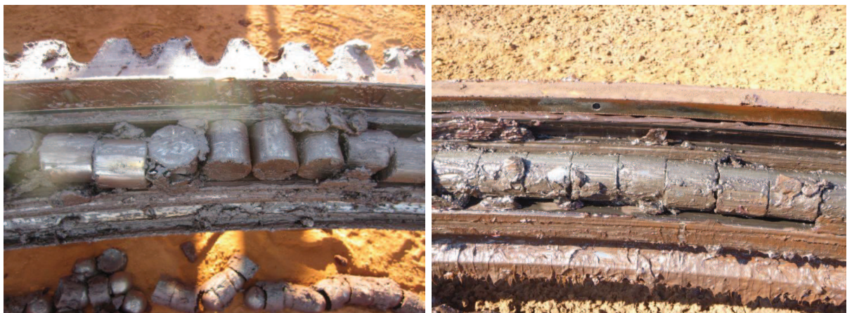
(a) Some roller elements are flipped
