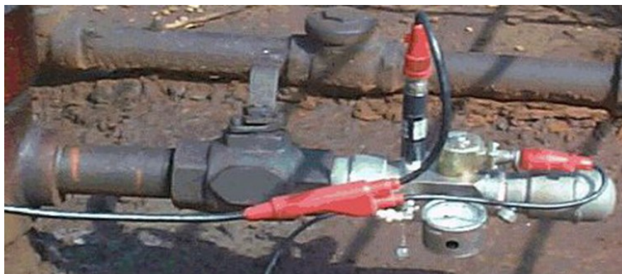
Figure 2.7: Gas gun installed on a well [36]
