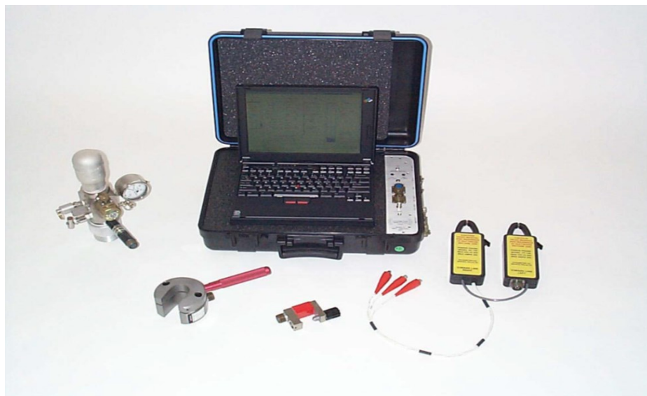
Figure 2.5: Portable well analyzer with sensors [36]
