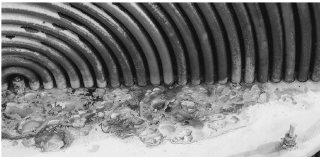
Figure 5-4 Pitting corrosion of an Alloy825 heat exchanger baffle exposed to seawater [31]
