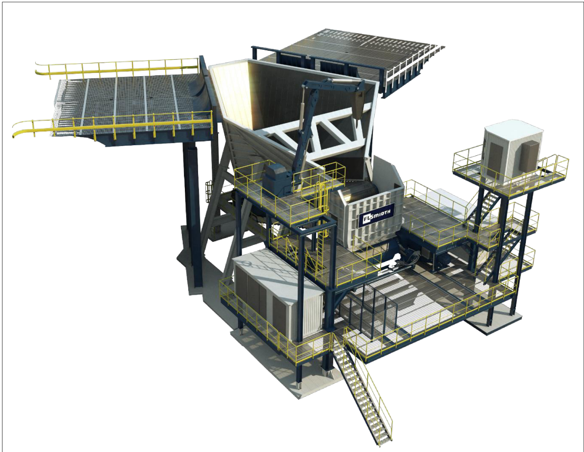
Figure 10: Semi-mobile In-Pit Crusher Station of FLSmidth (provided by FLSmidth)
