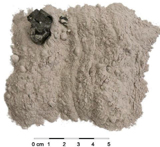
Figure 19: Disintegrated EAF slag that contains a minor number of lumpy pieces
