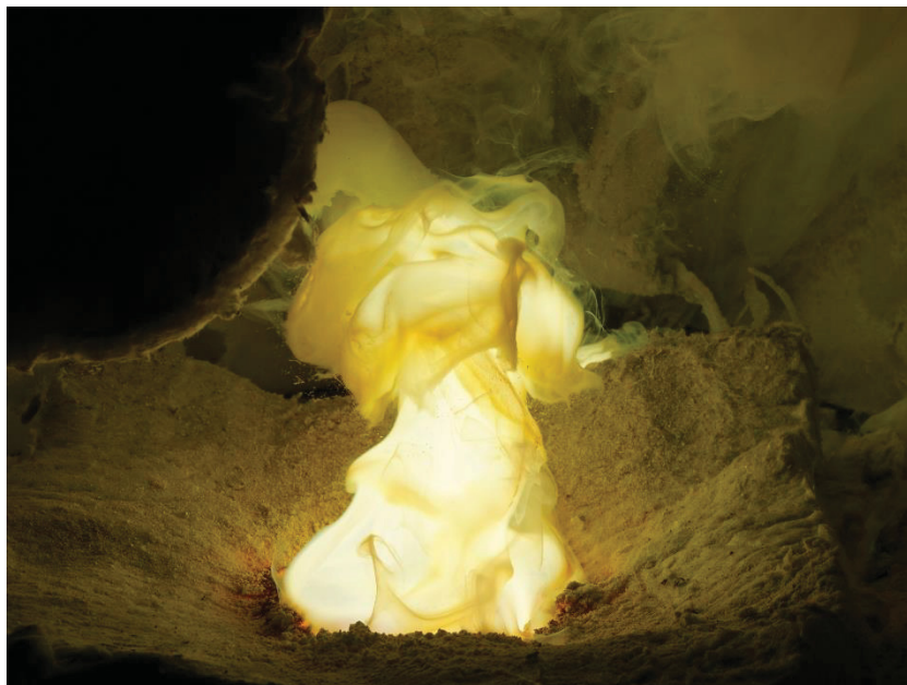
Figure 26: Re-oxidation of gaseous zinc to zinc oxide
