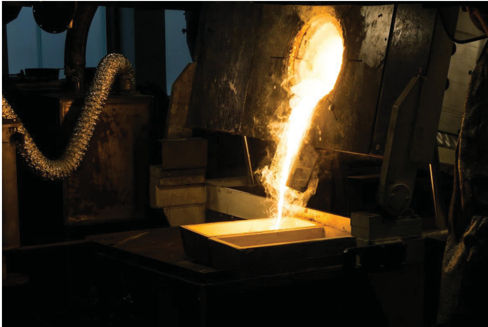
Figure 21: Tapping procedure after the pyrometallurgical treatment
