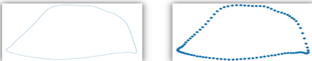
Figure 19: Original pump card and pump contour with boundary points
