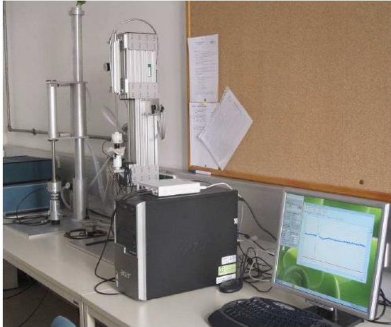
Figure 2.8: Photo showing the apparatus for ultrasonic laboratory velocity measurements (Pittino et al. 2016)
