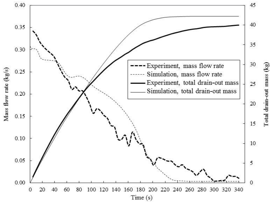
Figure 4.7 The total mass and the mass flow rate of the steel melt as drained from the nozzle are measured and plotted as functions of time [80]. They are then compared with the numerically simulated results.
