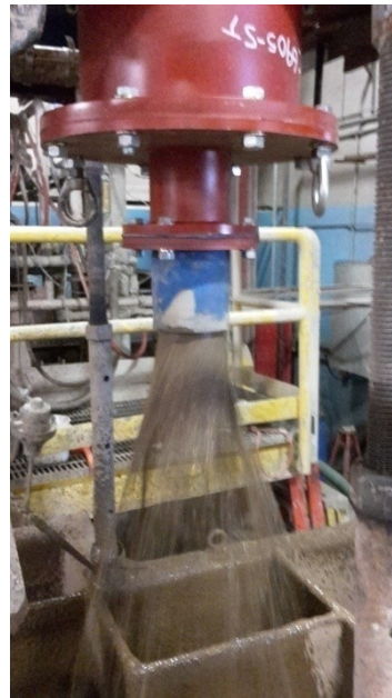
Figure 30: Spray discharge at 2.5 inch apex
