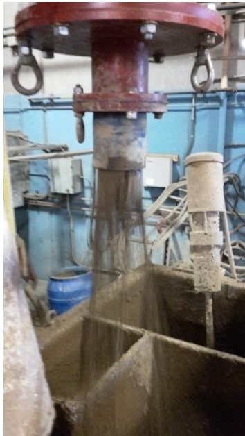
Figure 31: Normal discharge at 2.5 inch apex
