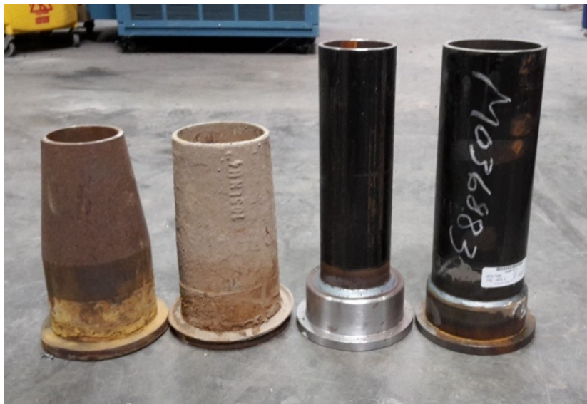
Figure 18: Vortex finders f.l.t.r.: 3 inch short, 4 inch short, 3 inch long, 4 inch long
