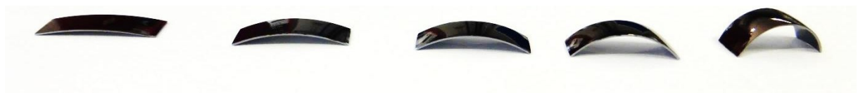
Fig. 4.17: Samples annealed for 15 min in a vacuum furnace at temperatures from 800 to 1000 °C from left to right, in steps of 50 °C.
