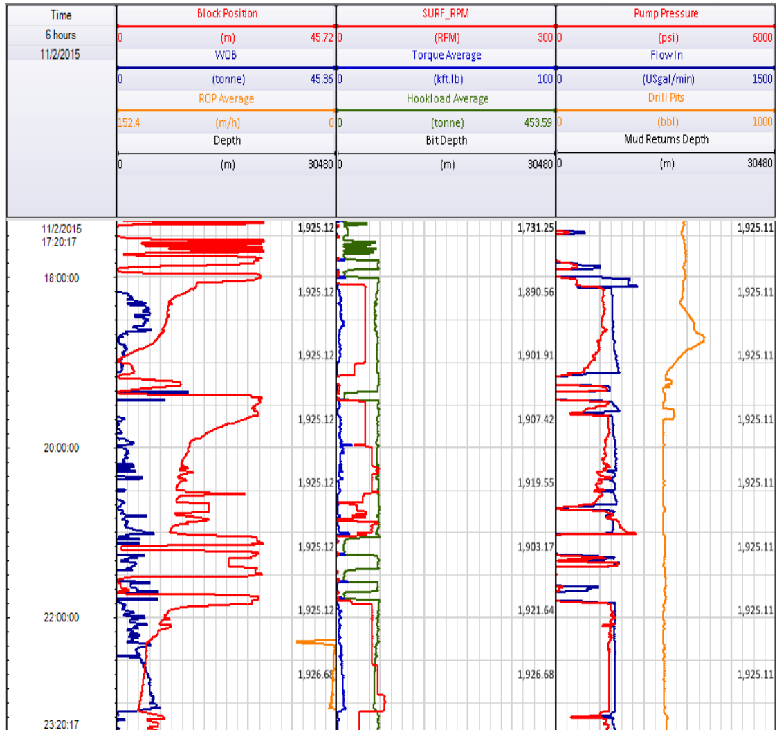
Figure 79: Drilling with casing (1790m-1920m)
