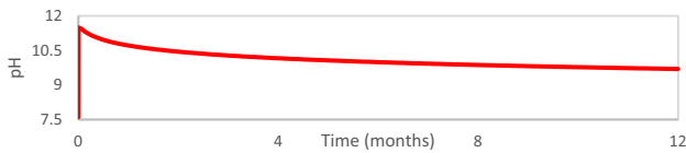
Fig. 9 Variation in pH (primary batch kinetic model based on initial system of case study 3 and assuming reactions of pyrite and pyrrhotite are at equilibrium)
