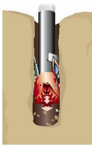
Figure 4 - Junk in the borehole - (2)
