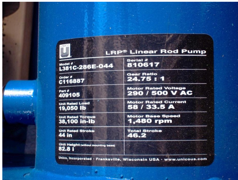
Figure 13: LRP model number example from Asset 9 Moldava Sud
