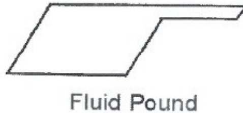
Figure 22: Dynamometer card shape of a fluid pound [27, p. 342]
