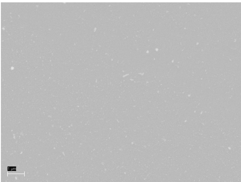
Figure 25: 18 at.% Ag of System B after annealing to 320°C for 1h
