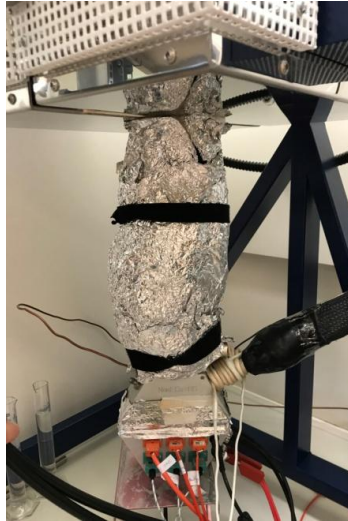
Figure 13: ProboStat insulated with glass wool and aluminium foil in operation.
