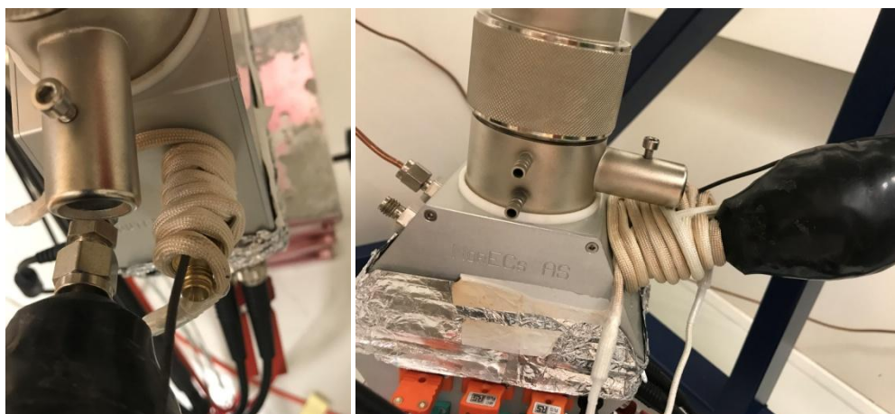
Figure 47: Heating cord mounted at the gas outlet (left), insulation of both the heating cord and the gas inlet (right).
