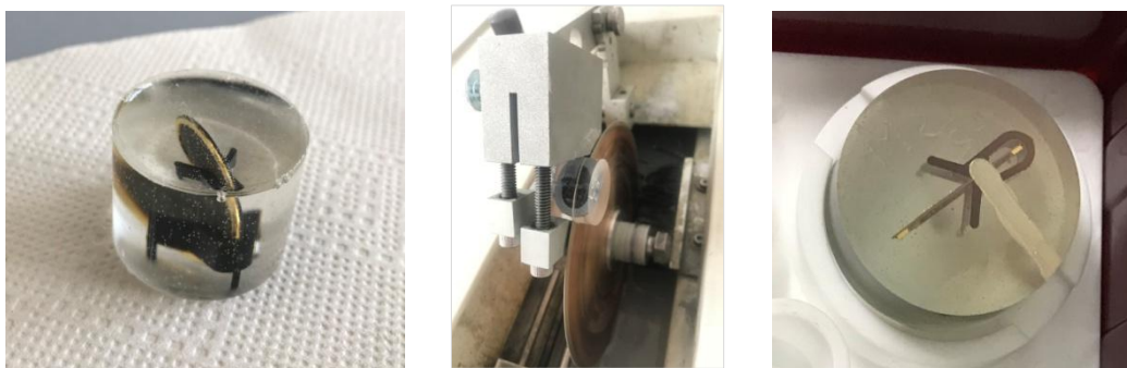
Figure 21: Embedded cell (left), cutting cell with saw (middle), contacted sample (right).
