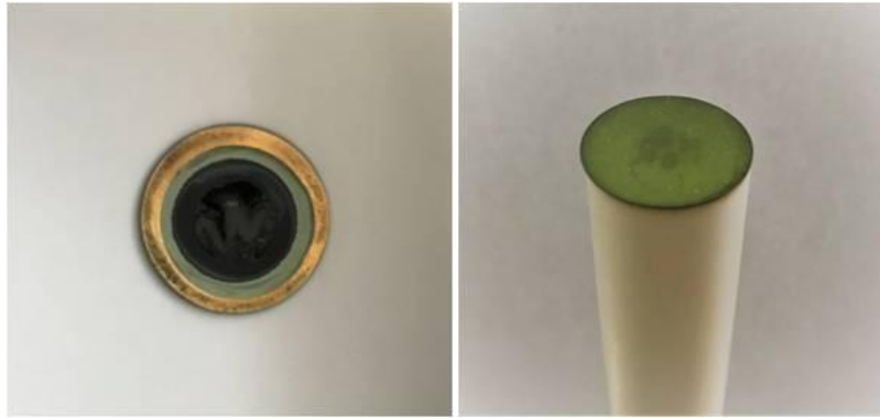
Figure 51: Cathode (left) and re-oxidised anode (right) of Cell 7 after disassembling.
