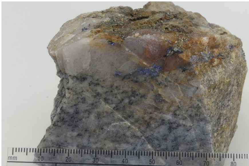
Figure 11: Hand specimen of Augengneiss with mineralized quartz joint (molybdenite and pyrite), sample 18PH5.
