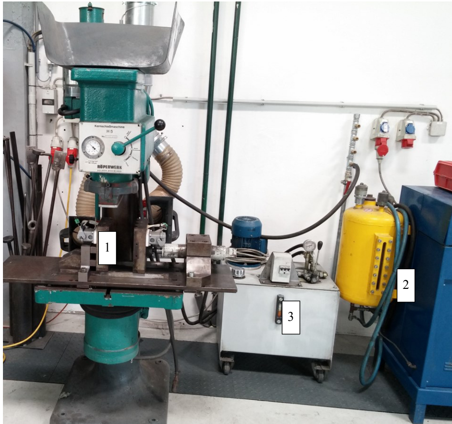
Figure 3-2: Core blowing machine of the type Röper H5 situated at the ÖGI in Leoben. (1) is a core box mounted on the machine table, (2) the gassing unit for Coldbox production and (3) a hydraulic unit for tool clamping.
