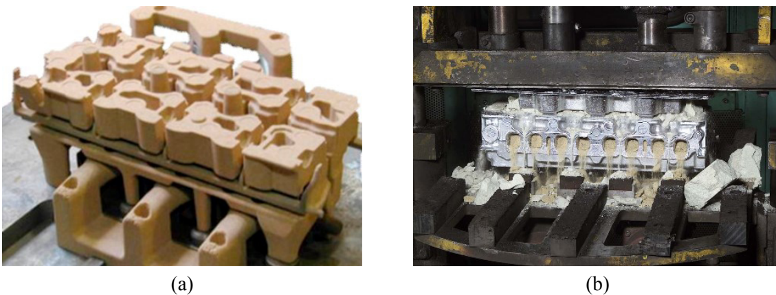
Figure 1-2 (a): Example of a sand core package to shape complex internal cavities of a car engine cylinder head prepared to be placed in a steel mould. (b): Cylinder head with cast-in sand cores during hammering for core removal (Nemak, 2005).
