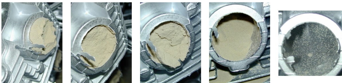
Figure 1-4: Picture sequence taken in 10 minute-steps starting after casting extraction from the mould (Picture 1) showing increasing, shell-wise core destruction with increasing time (Pictures 2-4) and the resulting channel after approximately 50 minutes from de-moulding 1 .
