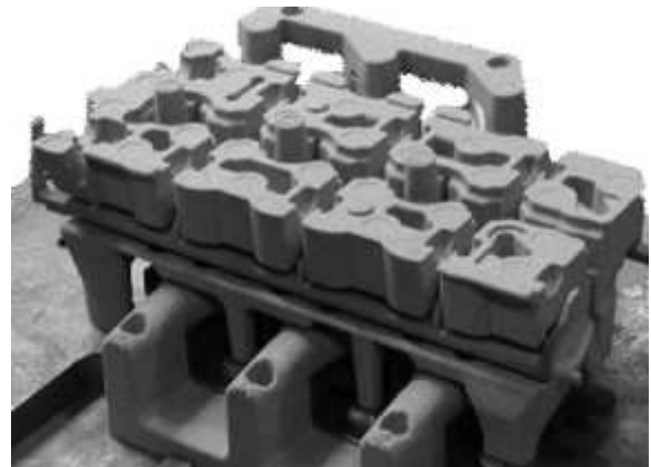
Fig. 2. Sand core package for an intricately shaped cylinder head prepared for casting by the Rotacast process (Gosch and Stika, 2005).
