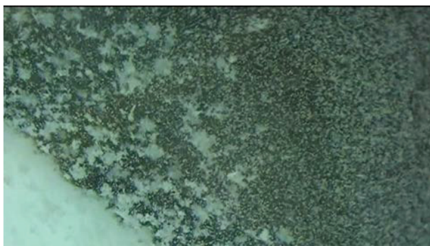
Fig. 3—Massive amount of crystal fragments that has formed only 16 s after a sliding down of a columnar area has started. Note that beside the larger fragments, the smaller fragments resemble the pre-existing equiaxed crystals and can thus not be distinguished.
