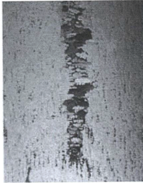
Fig. A21: Freckle of 2 mm diameter, observed in a Ni superalloy [M. C. Schneider A33].
