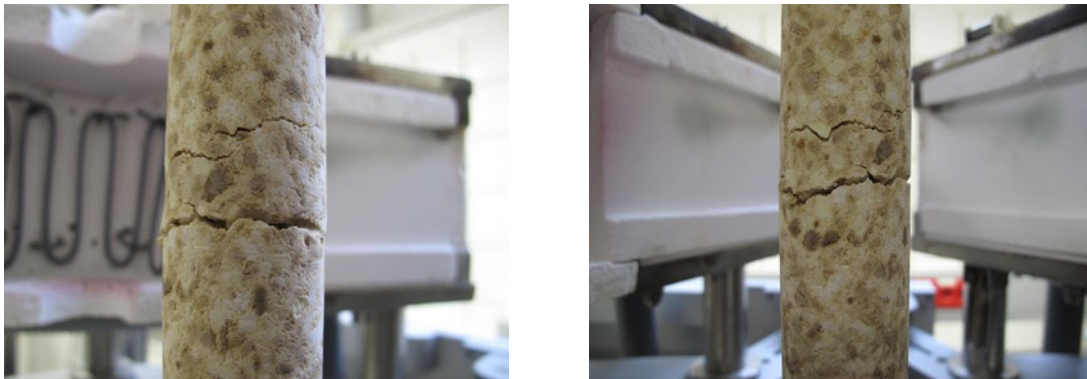
Figure 23: Magnesia-spinel specimen after creep testing at 1300 °C and 0.75 MPa.
