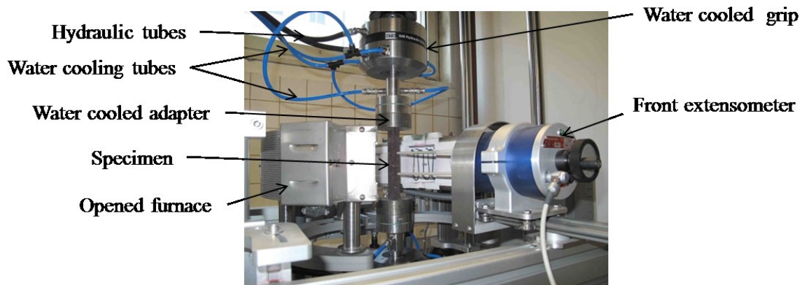
Figure 8: Tensile creep testing equipment; specimen, opened furnace and front extensometer.
