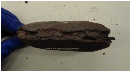
Figure 75: Changes of thickness of briquette due to segment wear
