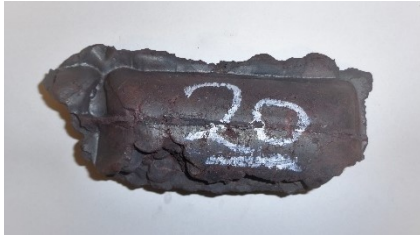
Figure 74: Briquette showing typical signs of segment wear
