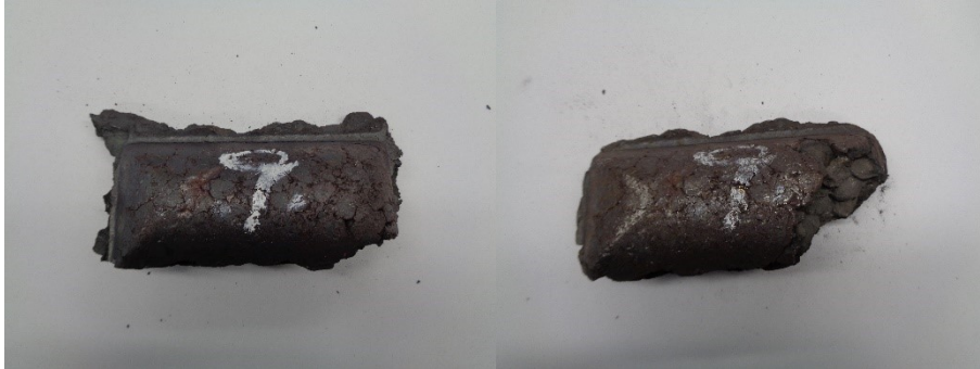
Figure 46: Briquette before and after tumble test; feed leg temperature of 1271 °F
