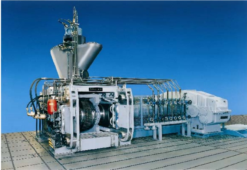
Figure 18: Briquetting press for lump ore and pellets, roller diameter 1 m [4]
