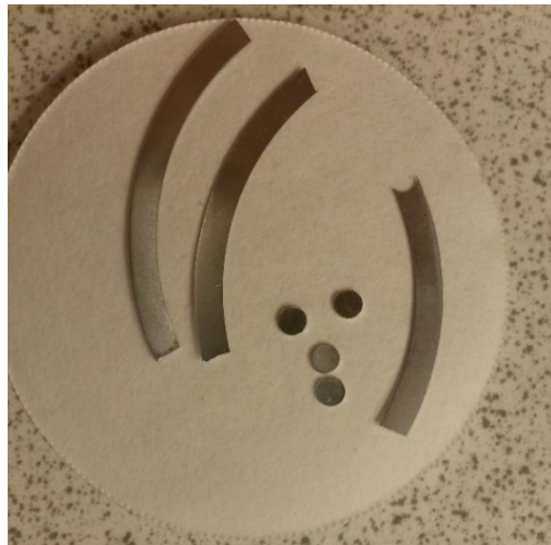
Fig. 7: Finished disk samples before electropolishing
