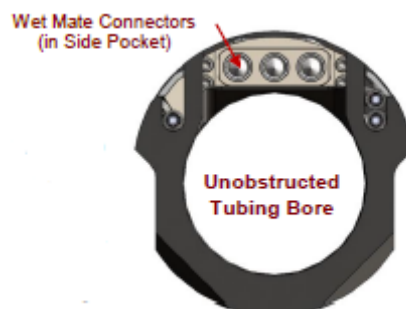
Figure 21: Wet mate connector and tubing bore [7]
