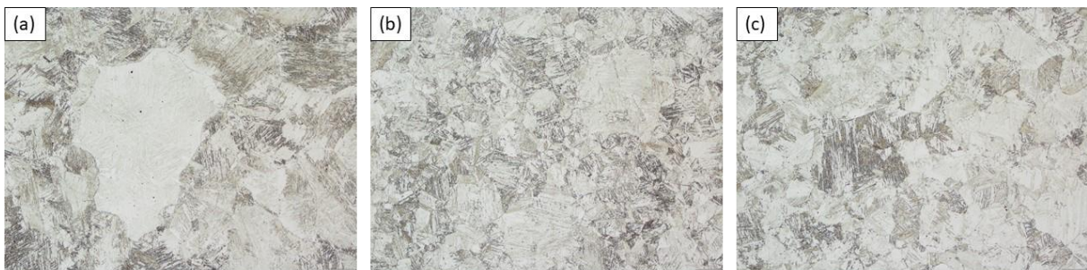
Figure 3-3: Microstructure after rotary hearth furnace, 50x, scale: 200µm; (a) Steel Grade A, (b) Steel Grade B and (c) Steel Grade C
