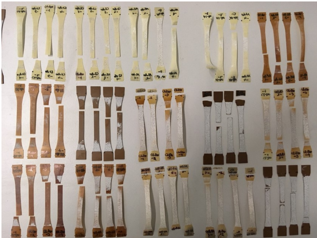
Figure A-5: Fractured specimens after the monotonic tensile test at room temperature and elevated temperatures.
