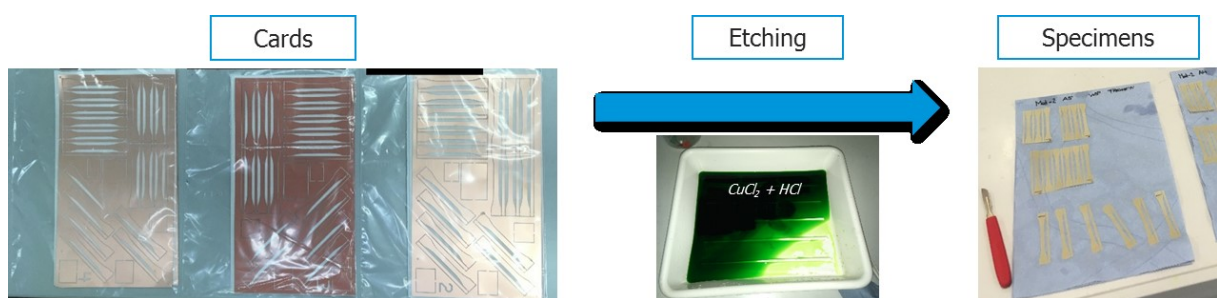
Figure 3-7: Final routed cards, the used etching solution and the specimens after performing the etching procedure.
