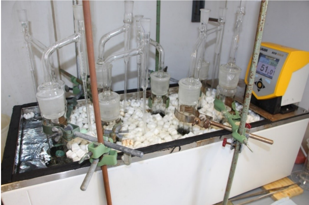
Figure 27: Illustration of the corrosion experimental setup
