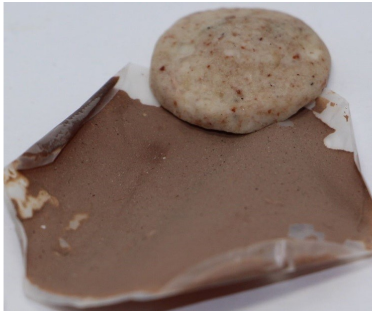
Figure 50: Untersberg formation tested with HCl @ 50°C
