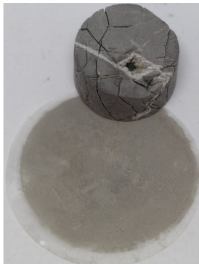
Figure 55: Hauptdolomit tested with HCl @ 50°C Figure 56: Hauptdolomit tested with lactic acid @ 50°C
