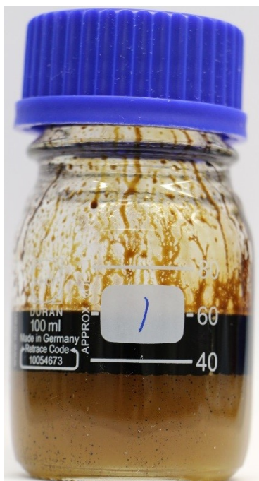
Figure 47: Emulsion breaker test using HCl in a 2:1 ratio
