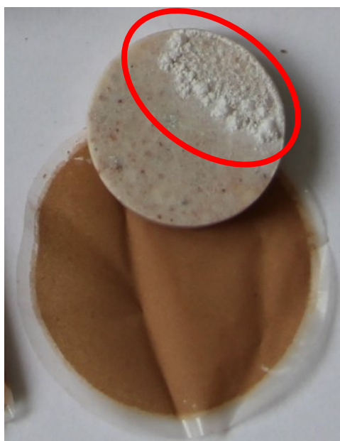
Figure 30: Reaction product formed during the limestone dissolving study using maleic acid
