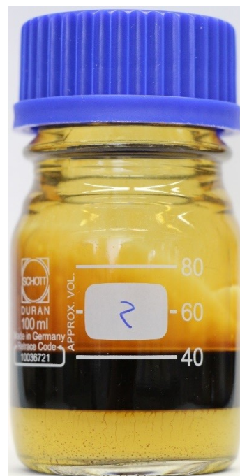
Figure 48: Emulsion breaker test using sulfamic acid in a 1:1 ratio
