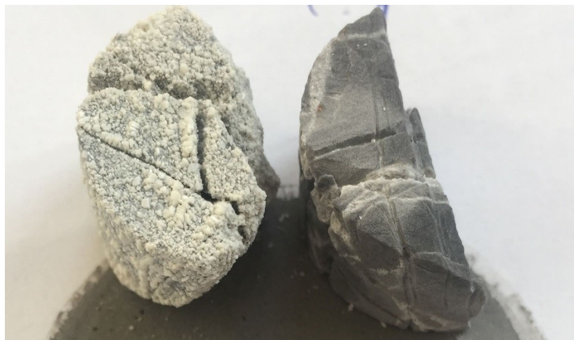
Figure 41: Reaction product formed during the dolomite dissolving study using maleic acid
