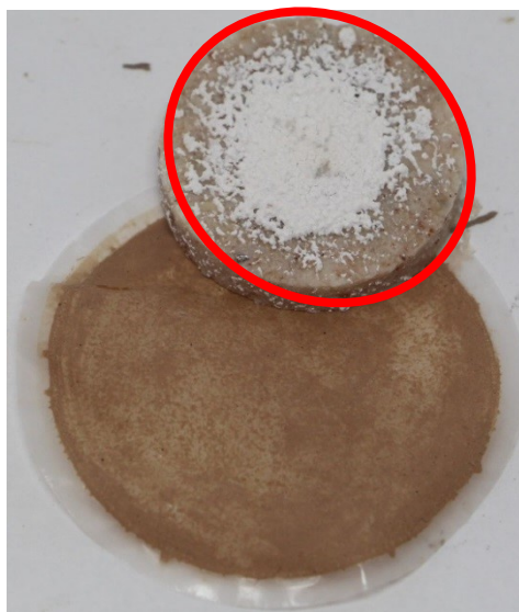
Figure 35: Reaction product formed during the limestone dissolving study using lactic acid
