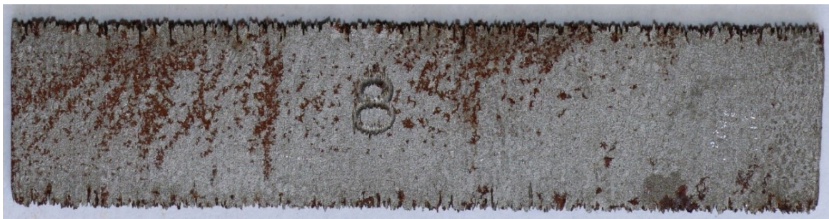
Figure 61: Visible alteration of the corrosion coupon tested with HCl after 24 hours
