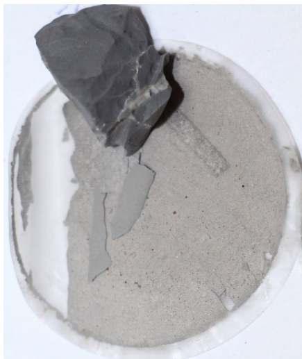
Figure 55: Hauptdolomit tested with HCl @ 50°C Figure 56: Hauptdolomit tested with lactic acid @ 50°C
