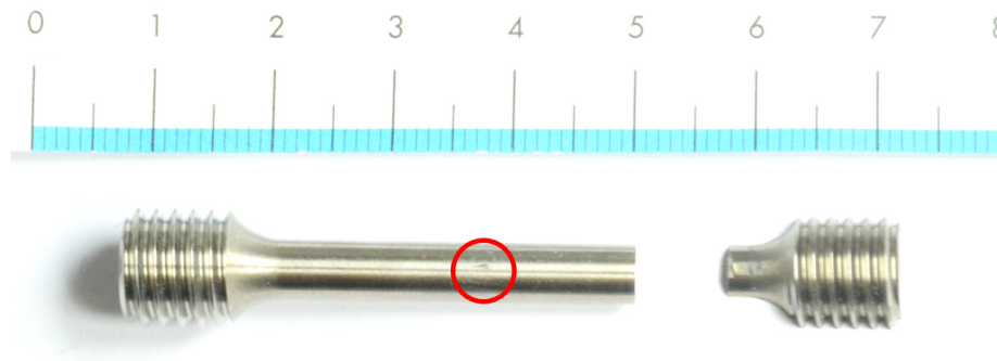
Figure 4.12: Photos of a sample that broke far from the centre of the testing length. The red circle indicates a nick in the surface.
