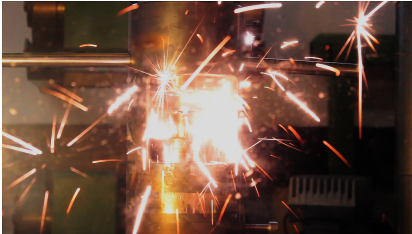
Figure 2.3.: Photo of an explosion during the HPT process. No changes of the microstructure are detectable compared to specimens which did not explode. Drying the used powders prior to deformation could reduce the probability of explosions.
