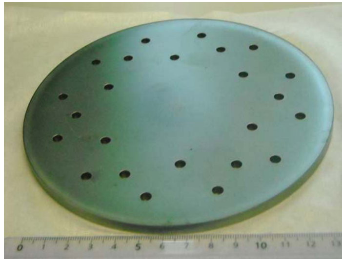
Figure 4.2: Molybdenum “mosaic” target with holes for the alloying-elements-inserts.
