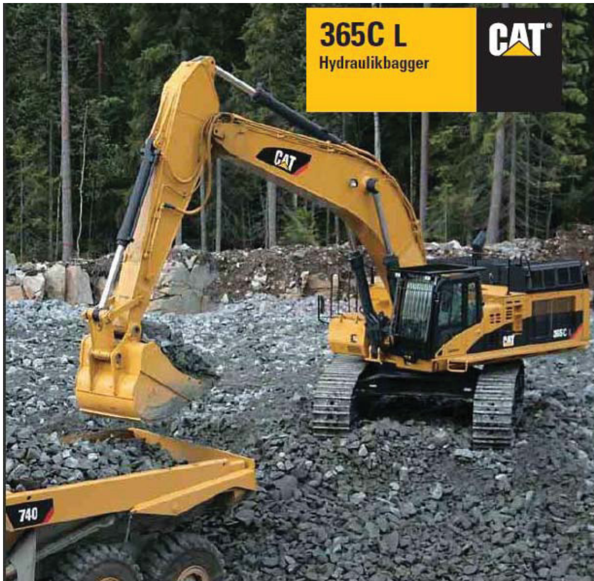
Figure 25: CAT 365C L pull shovel excavator
