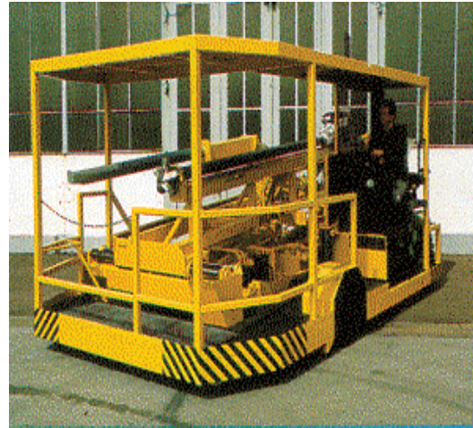
fig. 41: taphole changing device 76
