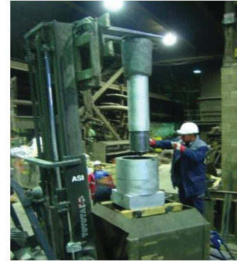
fig. 65: insertion of taphole to surround block
