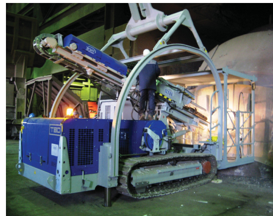
fig. 45: backwrecking of the worn taphole and cleaning of taphole channel
