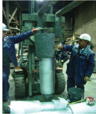
fig. 64: covering of the conical part of C-Type
