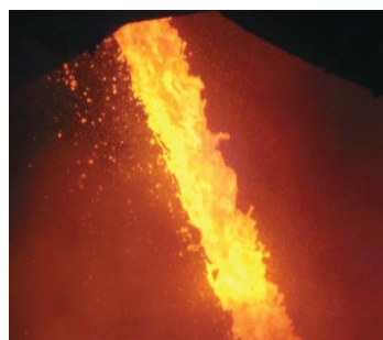
fig. 73: tapping stream common taphole
