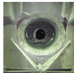
fig. 68: breakout of old surround block
