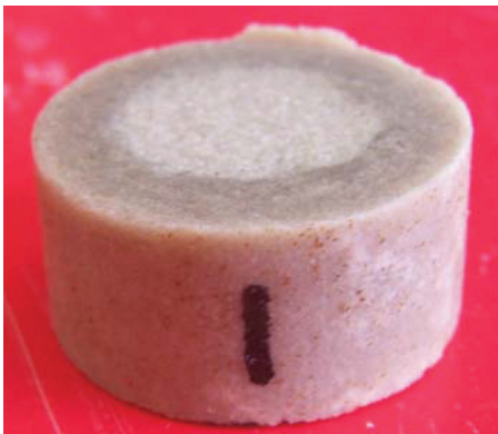
Figure 102: 5% clay – top 0.5inch of the consolidated sample
