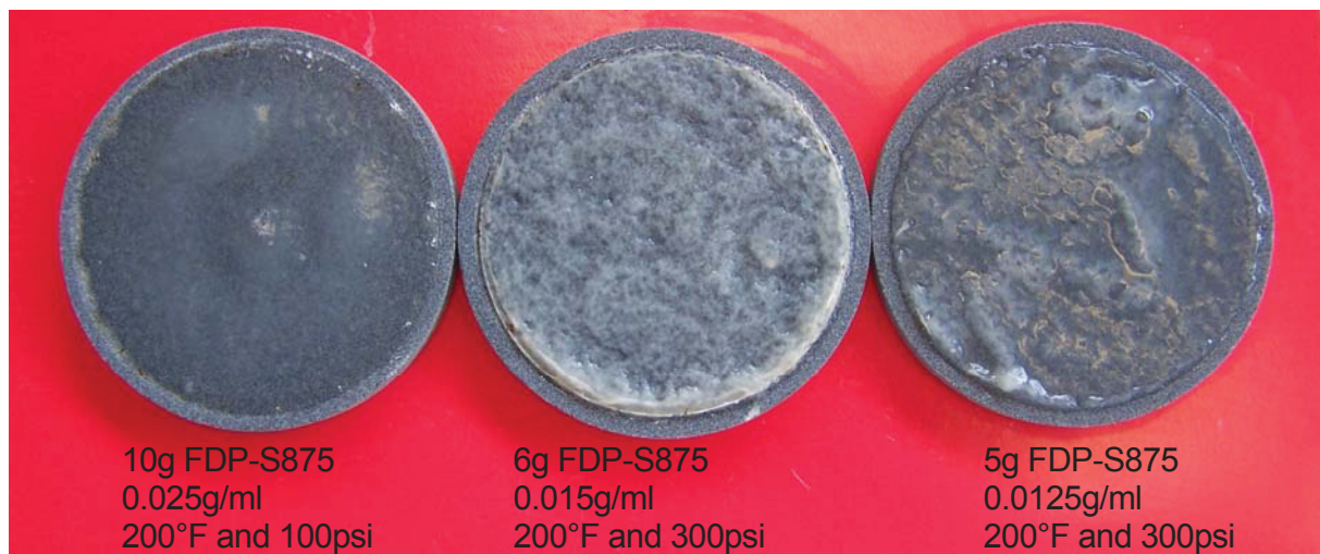
Figure 35: FDP-S875 on 20 micron sand discs
