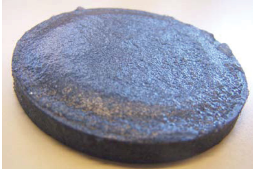
Figure 73: Filter cake made from the rigid Pam gel
