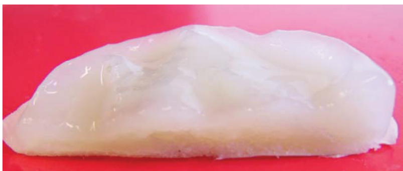
Figure 29: Filter cake showing jelly-like texture at surface and grainy texture on bottom
