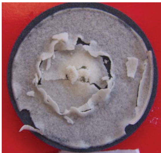
Figure 57: 1g FDP-S875 2min soaking time in 80°F brine
