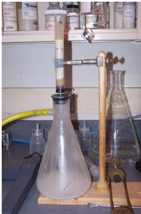
Figure 91: Testing of consolidation ability of resin/FDP-S875 mixture
