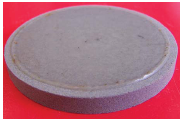
Figure 78: 0.75g FDP-S875 on a 10 micron filter disc
