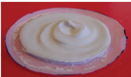
Figure 68: Baracarb filter cake on 11 micron Whatman filter paper
