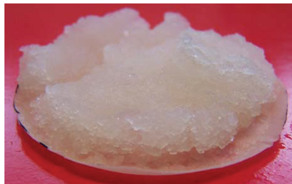
Figure 26: wet FDP-S875 filter cake on 8 micron filter paper (RT)
