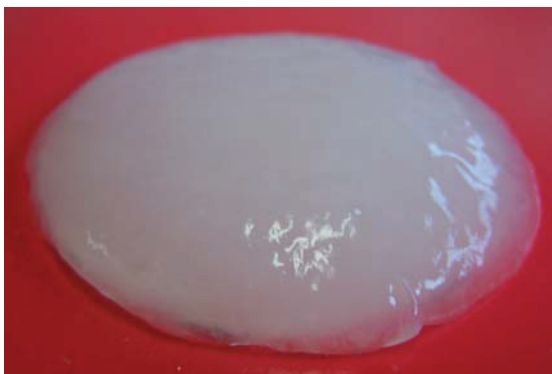
Figure 25: wet FDP-S875 filter cake on 8 micron filter paper (160°F)
