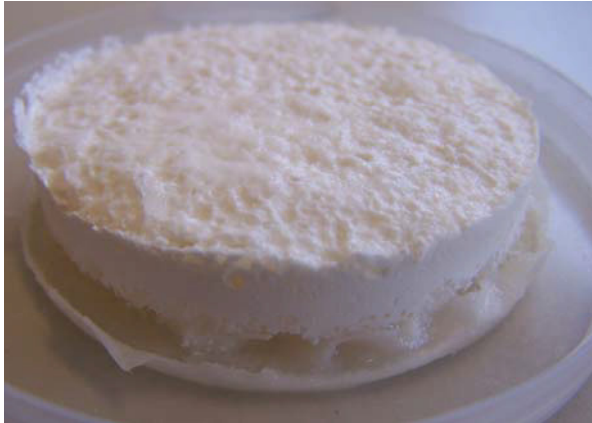
Figure 87: wet FDP-S875/resin filter cake after HCl treatment
