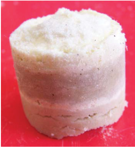
Figure 100: 0.5% clay – S875 filter cake and previously consolidated top plug
