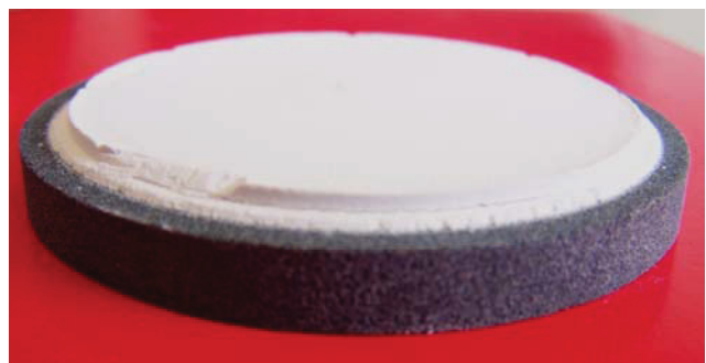
Figure 69: Baracarb filter cake on 20 micron ceramic filter disc
