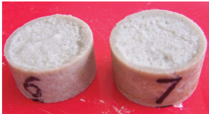
Figure 103: 5% clay – bottom 1inch of the consolidated sample
