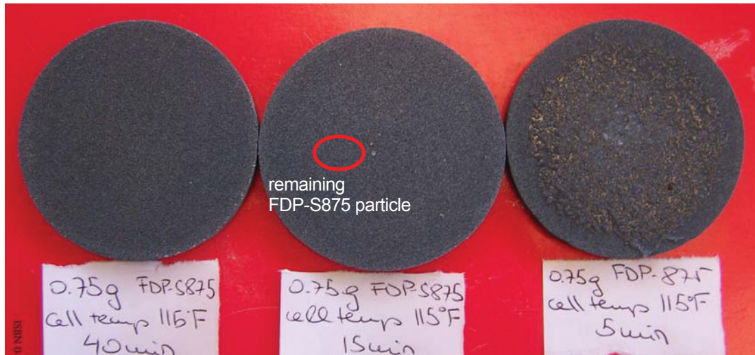
Figure 56: Various soaking times of 0.75g FDP-S875 in 115°F 6%KCl brine
