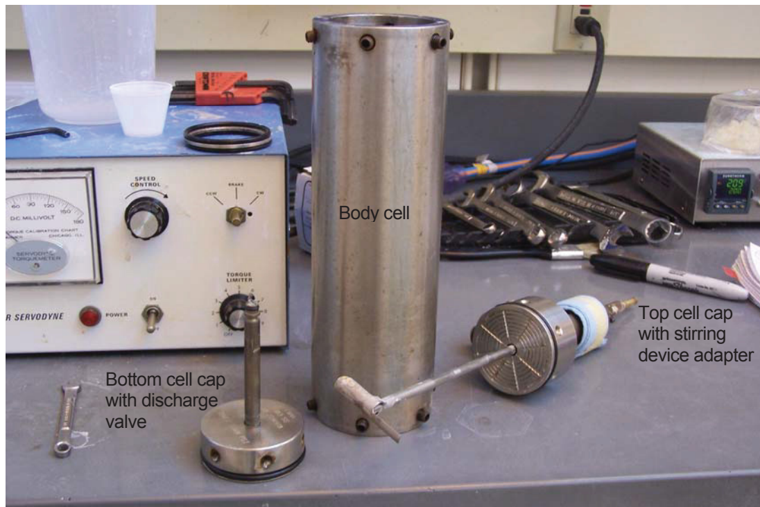
Figure 16: Parts of the HPHT Filter Press
