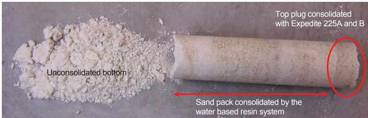
Figure 98: Consolidated sand pack
