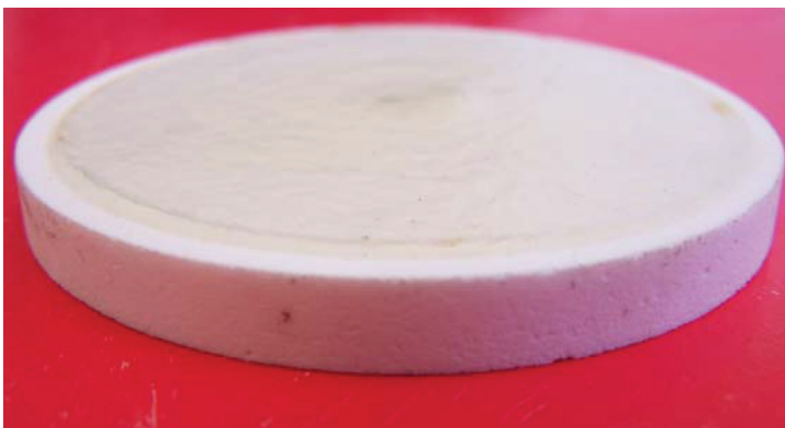
Figure 77: 0.75g FDP-S875 on a 5 micron filter disc
