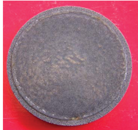
Figure 80: 0.75g FDP-S875 on a 35 micron filter disc – top view
