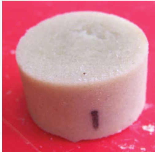
Figure 101: 0.5% clay – top 0.5inch of the consolidated sample
