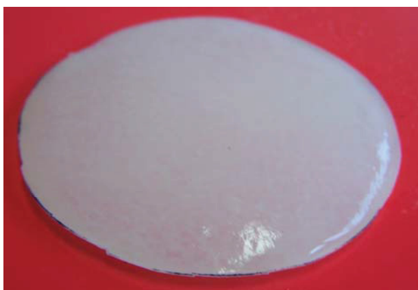
Figure 23: dry FDP-S875 filter cake on 8 micron filter paper (180°F)
