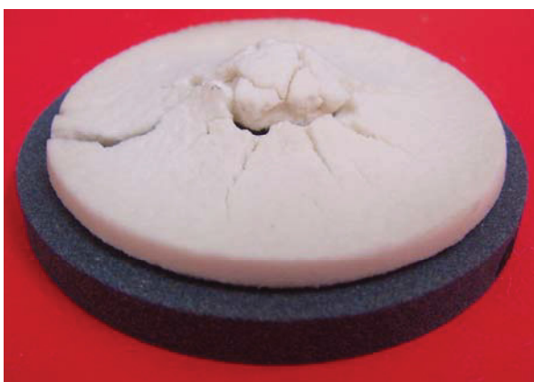
Figure 45: 6g FDPS-875 at 135°F (0.015g/ml) – no seal created
