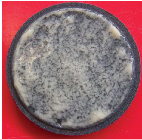
Figure 94: Filter cake built during HPHT fluid loss test in water based resin system
