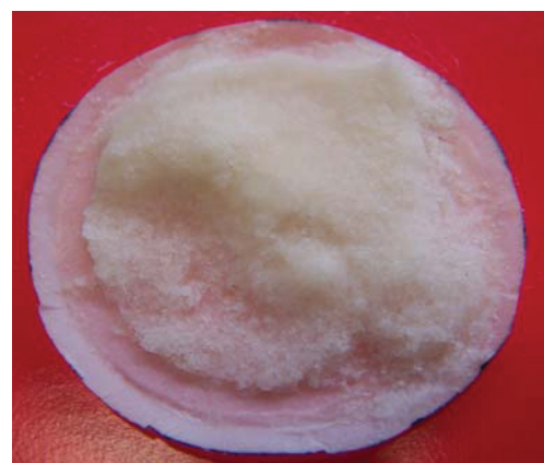
Figure 24: dry FDP-S875 filter cake on 8 micron filter paper (RT)
