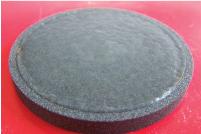
Figure 79: 0.75g FDP-S875 on a 35 micron filter disc
