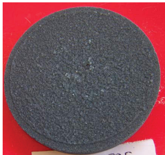
Figure 58: 1g FDP-S875 34min soaking time RT brine
