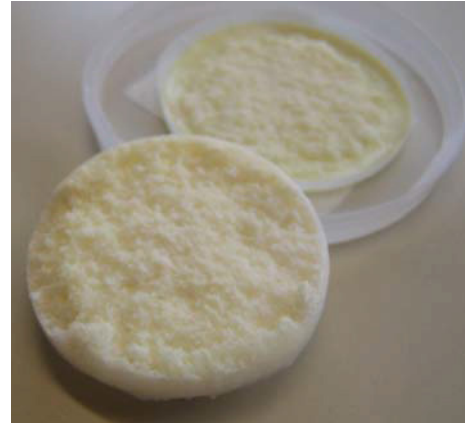
Figure 88: wet FDP-S875/resin filter cake after HCl treatment
