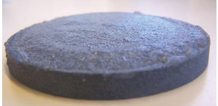
Figure 74: Filter cake made from the rigid Pam gel – side view
