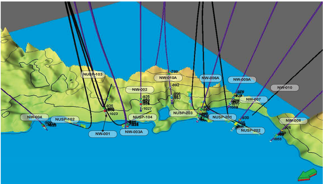
Figure 5.2: Ten production wells and six prospected storage wells are intersecting Nußdorf reservoir. The storage wells are planned to be drilled from two cluster well sites.
