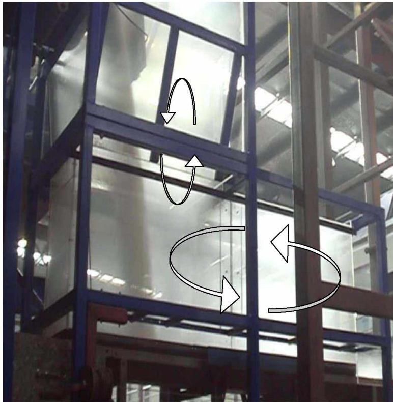
Picture 61: Turbulence in the setup with the reduced drop height and the gate open
