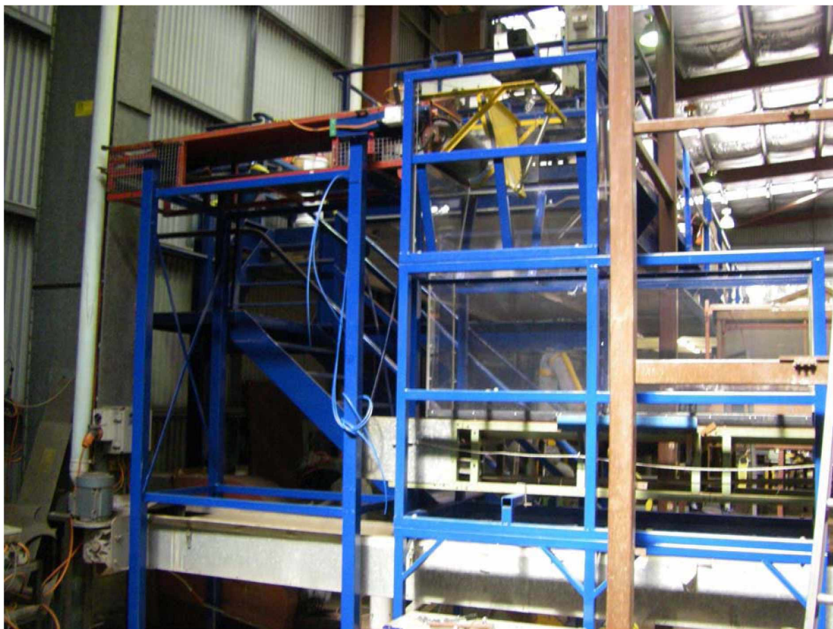
Picture 27: Setup for the reduced drop height without the hopper
