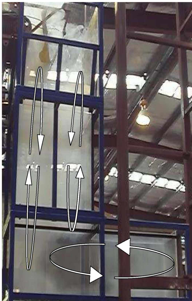
Picture 60: Turbulence in the setup with the full drop height and the gate open
