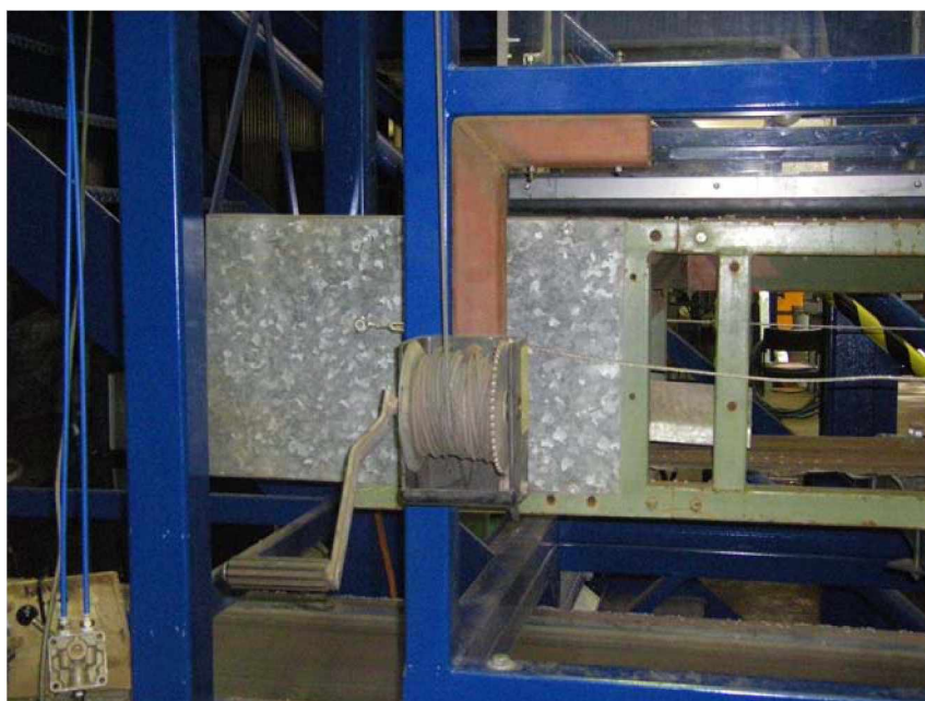
Picture 23: Crank handle with steel wire to fix the impact plate
