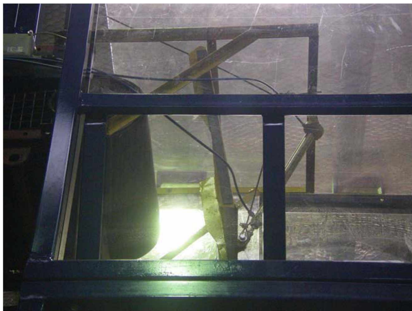
Picture 22: The impact plate in position wired up with air hoses and the steel wire
