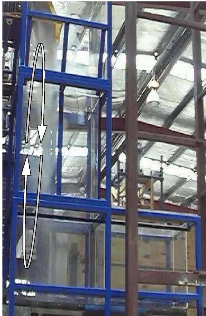
Picture 37: Main turbulence in the left side of the vertical part of the rig
