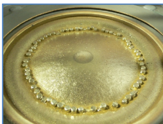
Figure 4-1: Addition of 48 Ti pieces, in a row, in order to achieve a \text{Ti}_{0.5}\text{Al}_{0.5}\text{N} films.
