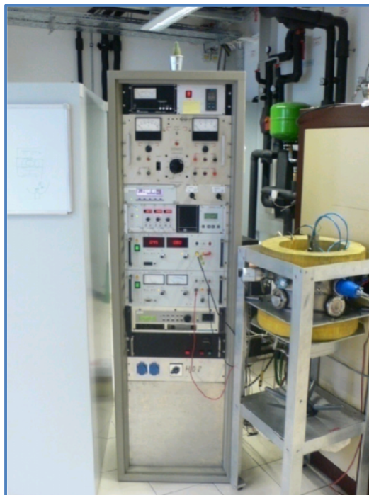
Figure 3-2: Picture of the reactive magnetron sputtering system used in this thesis.
