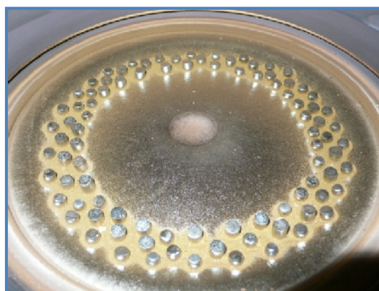
Figure 4-2: Addition of 48 Ti pieces, evenly distributed, in order to achieve a \text{Ti}_{0.75}\text{Al}_{0.25}\text{N} films.
