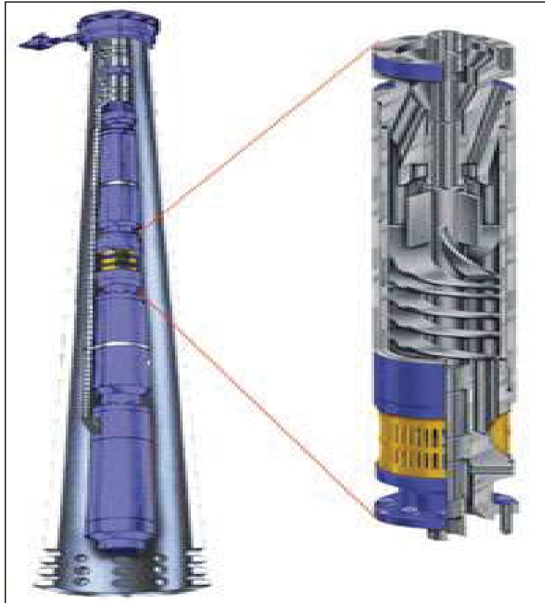
Figure 3-6: Centrifugal Gas Separator [8]
