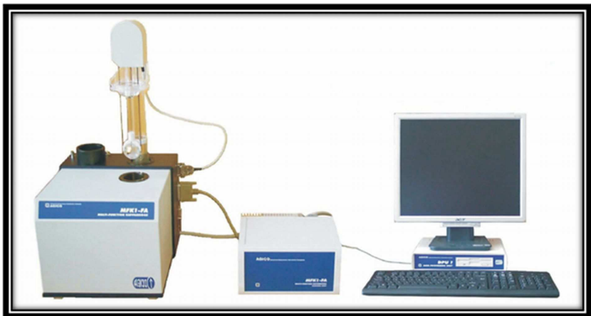
Figure 15: Geofyzika MFK1-FA Kappabridge from AGICO (from AGICO MFK1-FA Kappabridge User's Guide).
