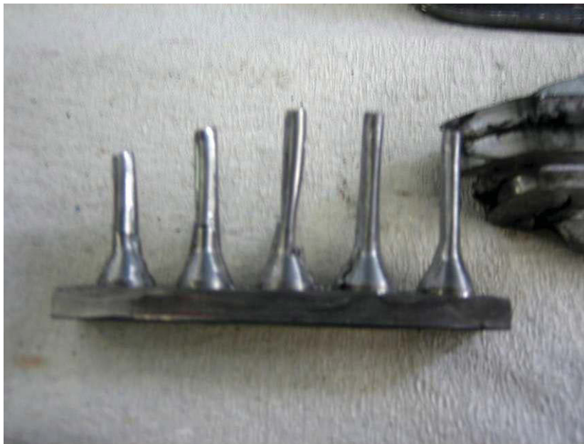
Figure 35: Tubular plate with five spines extruded in the laboratory
