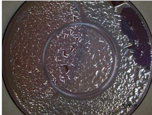
Fig. 4.21: Delamination of the coating with 5.8 at% after tribo-testing at 600 °C.
