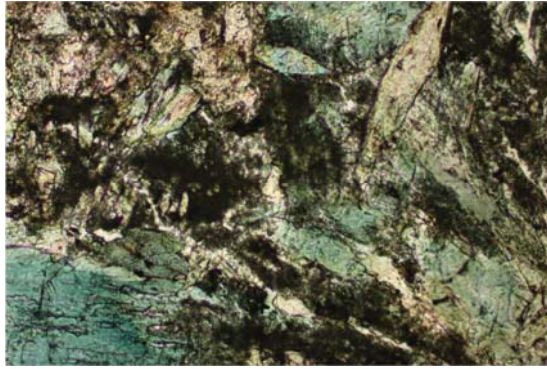
Figure 3-44: Tremolites and epidotes - transmitted light (10 times extension, length of the picture correlates to 3.6 millimeters)
