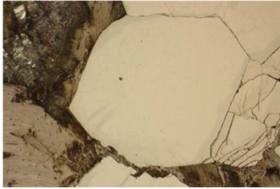
Figure 3-34: Almandine - reflected light (10 times extension, length of the picture correlates to 3.6 millimeters)
