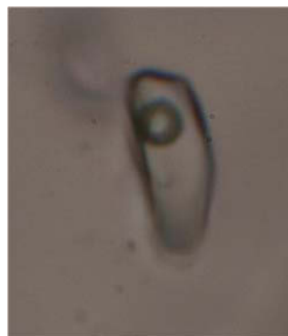
Figure 3-31: Fluid inclusion of the quartzitic fissure (length of the picture correlates to 0.18 mm)
