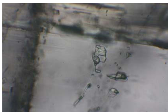
Figure 3-47: Fluid inclusion trapped in an amphibole (length of the picture correlates to 0.8 mm)
