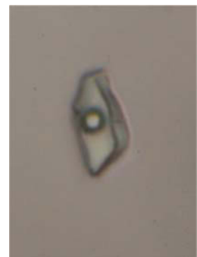
Figure 3-30: Fluid inclusion of the quartzitic fissure (length of the picture correlates to 0.12 mm)
