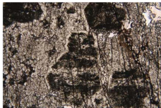
Figure 3-12: Brittle ductile deformation of garnets in transmitted light (10 times extension, length of the picture correlates to 3.6 millimeters)
