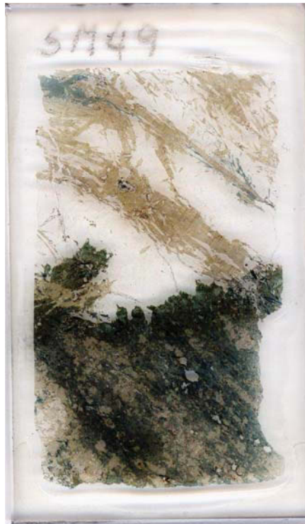
Figure 3-41: Scanned thin section SM49 (length of the picture correlates to 2.8 x 4.8cm)
