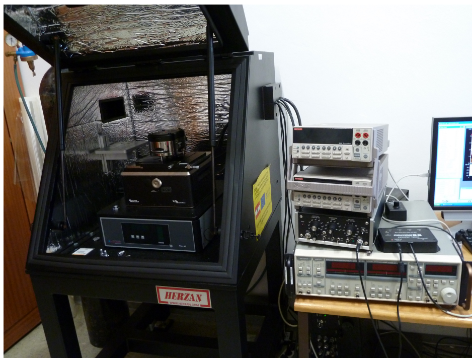
Figure 3.2: Asylum Research MFP-3D™ system at the Institute of Physics in Leoben. Right to the AFM from bottom to top are a Lock-In Amplifier from Stanford Research Systems, an external current preamplifier from DL Instruments and two Keithley 2400 sourcemeters to apply higher sample bias than the MFP can apply.
