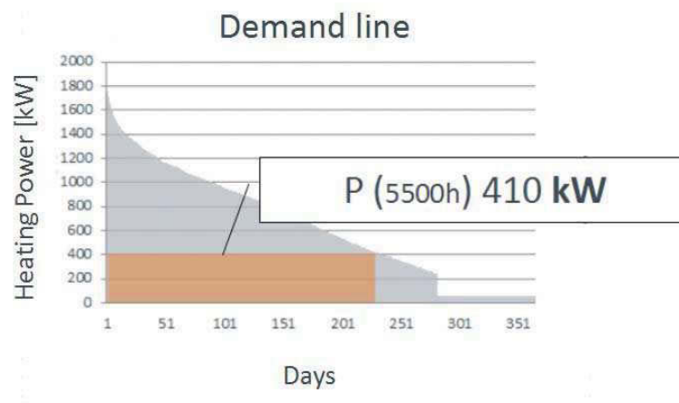
Figure 159: Case 1 - No storage included – Demand line and heat energy support [own illustration]
