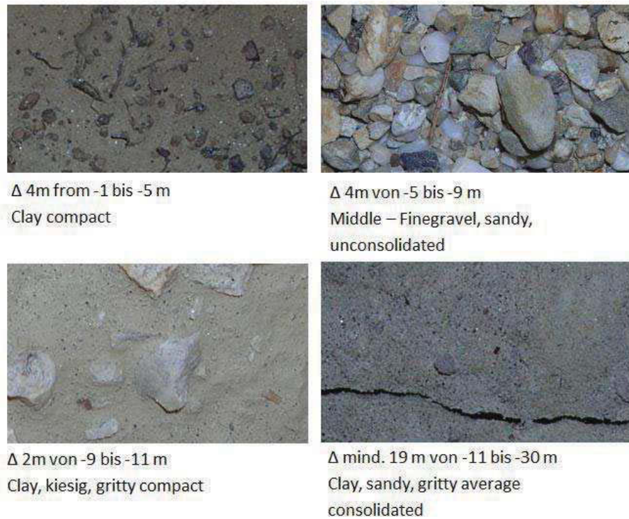
Figure 208 Sediment cores from the test well in St. Georgen bei Obernberg am Inn (~1km distance). [Own photography]
