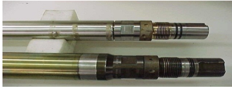
Fig.77: Difference in electronics module housing thickness between a normal (upper) and an HP/HT acoustic tool (lower) [90]
