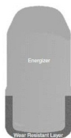
Fig.57: Cross-section of a modern bi-material seal [52]
