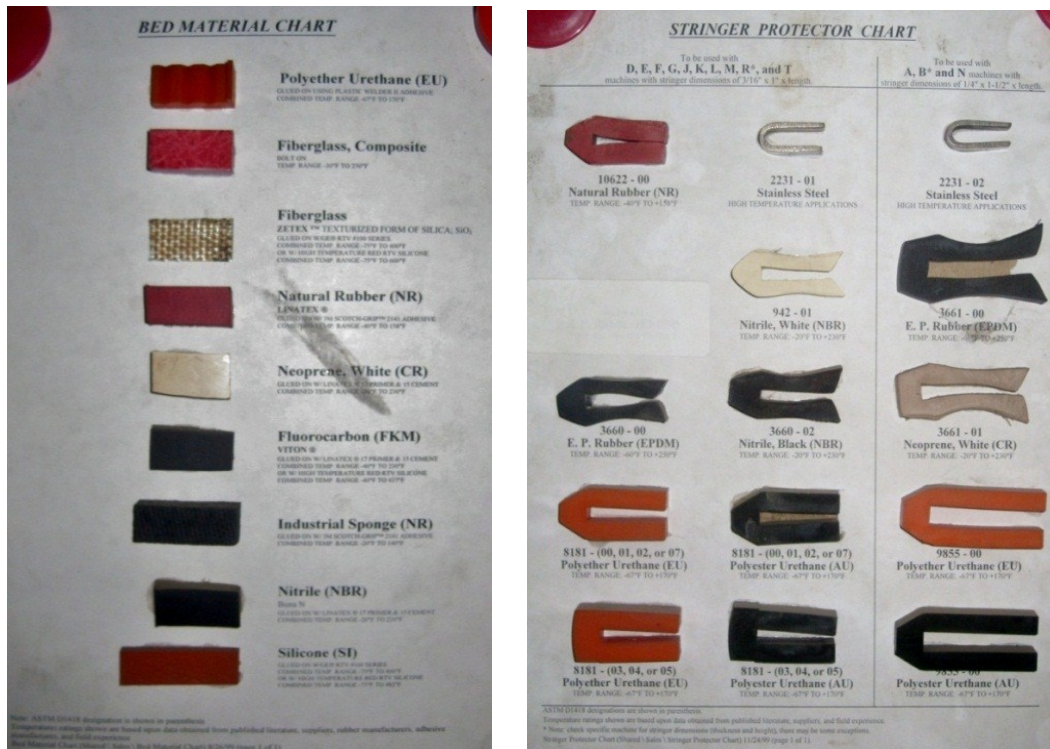
Fig.62: Bed material probes (left) and stinger protector probes (right) with allowed temperatures
