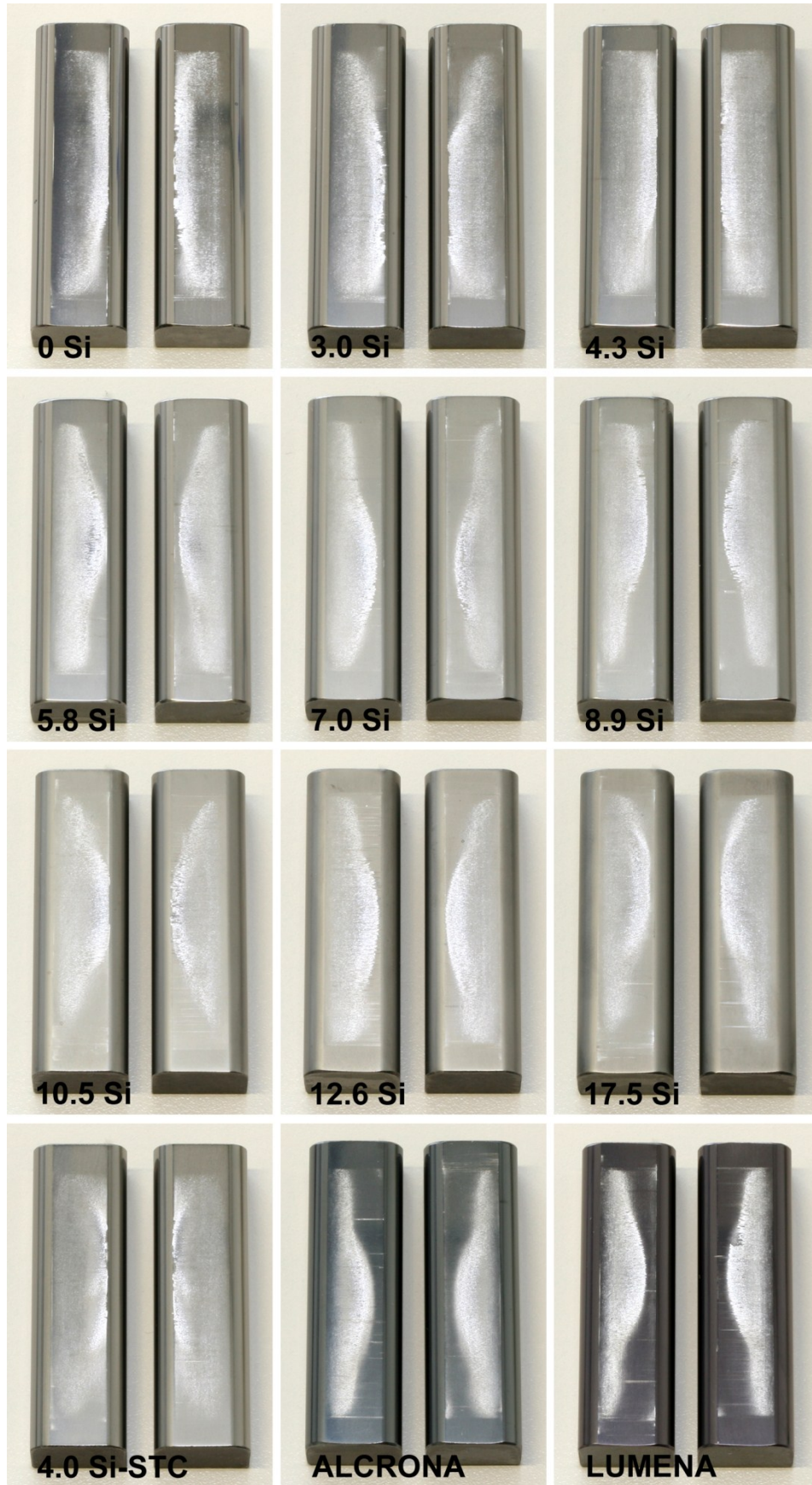
Figure 4.26: Drawing jaws after hardware test. Each pair was tested 5 times.
